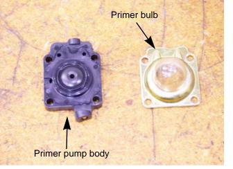
6. Inspect the primer pump body for dirt and/or varnish. See Figure 5.27.
